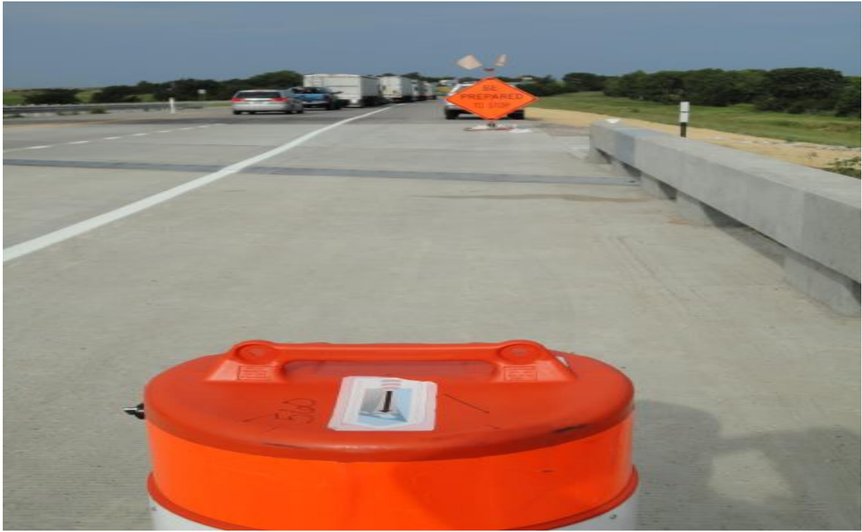
Figure 20. iCone test setup on US-50 near Newton, KS.
