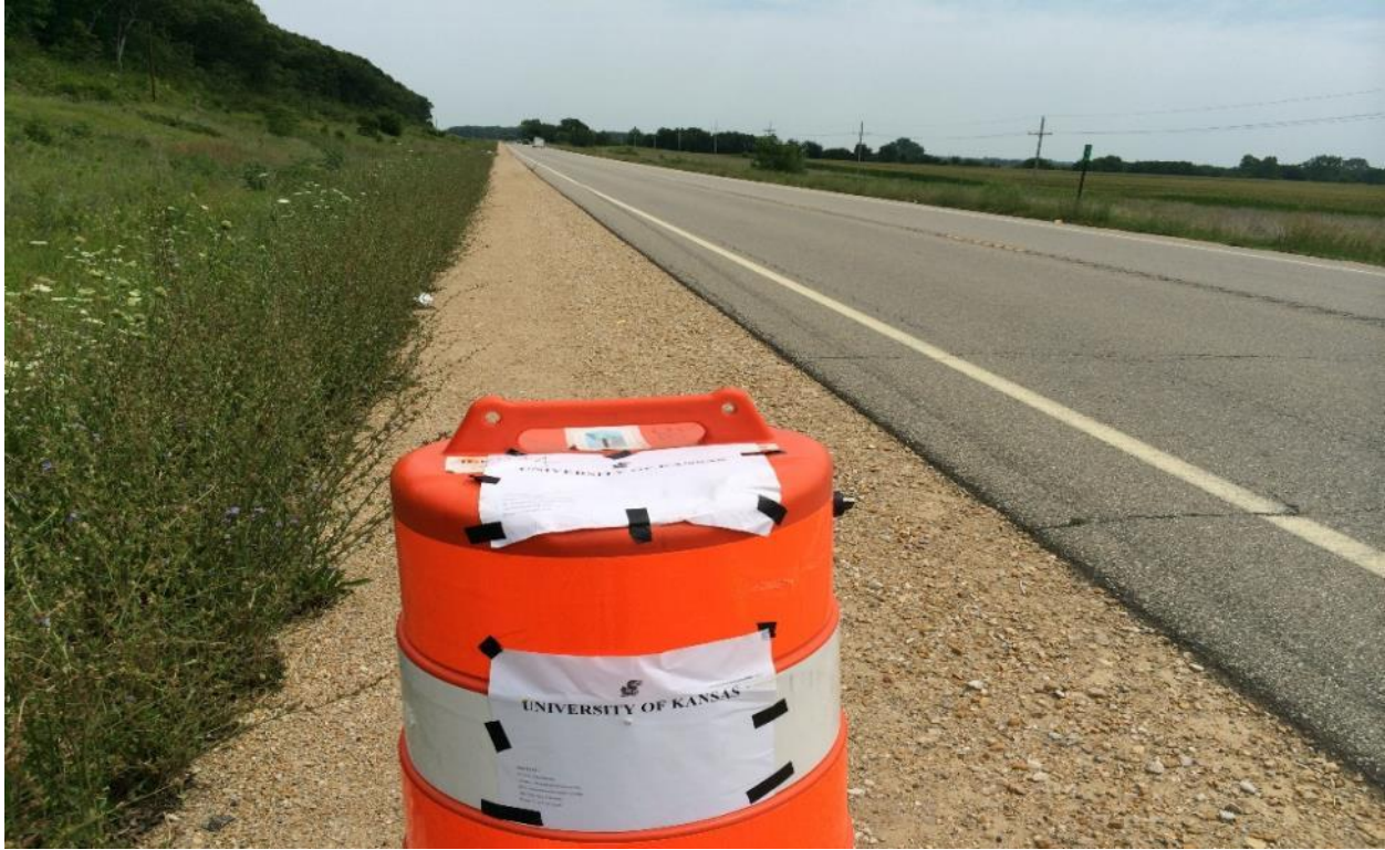
Figure 16. iCone test setup on US-24 near Williamstown, KS.
